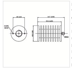
RF Solution offer a wide selection of Coaxial Fixed Termination (Dummy Load) for global customers. CT-30W-RA3857-SK-18G is a Coaxial Fixed Termination (Dummy Load) in Frequency Range of DC~18.0 GHz. It is made of high quality materials under a high standard, the Connector Type of this product is SMA-F (K), VSWR Max is 1.35 and Impedance is 50  $\Omega$ . The component has a good working performance and stability, it is ideal for handling a Power of 30 W.
