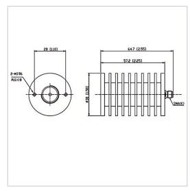
RF Solution offer a wide selection of Coaxial Fixed Termination (Dummy Load) for global customers. CT-30W-RA3857-SK-12.4G is a Coaxial Fixed Termination (Dummy Load) in Frequency Range of DC~12.4 GHz. It is made of high quality materials under a high standard, the Connector Type of this product is SMA-F (K), VSWR Max is 1.30 and Impedance is 50  $\Omega$ . The component has a good working performance and stability, it is ideal for handling a Power of 30 W.
