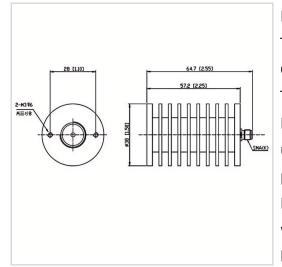
RF Solution offer a wide selection of Coaxial Fixed Termination (Dummy Load) for global customers. CT-30W-RA3857-SK-10G is a Coaxial Fixed Termination (Dummy Load) in Frequency Range of DC~10.0 GHz. It is made of high quality materials under a high standard, the Connector Type of this product is SMA-F (K), VSWR Max is 1.30 and Impedance is 50  $\Omega$ . The component has a good working performance and stability, it is ideal for handling a Power of 30 W.
