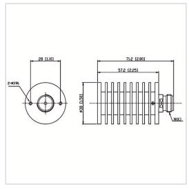
RF Solution offer a wide selection of Coaxial Fixed Termination (Dummy Load) for global customers. CT-30W-RA3857-NK-8G is a Coaxial Fixed Termination (Dummy Load) in Frequency Range of DC~8.0 GHz. It is made of high quality materials under a high standard, the Connector Type of this product is N-F (K), VSWR Max is 1.30 and Impedance is 50  $\Omega$ . The component has a good working performance and stability, it is ideal for handling a Power of 30 W.
