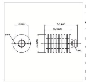
RF Solution offer a wide selection of Coaxial Fixed Termination (Dummy Load) for global customers. CT-30W-RA3857-NK-6G is a Coaxial Fixed Termination (Dummy Load) in Frequency Range of DC~6.0 GHz. It is made of high quality materials under a high standard, the Connector Type of this product is N-F (K), VSWR Max is 1.25 and Impedance is 50  $\Omega$ . The component has a good working performance and stability, it is ideal for handling a Power of 30 W.
