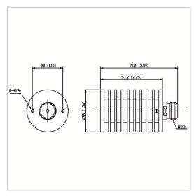
RF Solution offer a wide selection of Coaxial Fixed Termination (Dummy Load) for global customers. CT-30W-RA3857-NK-3G is a Coaxial Fixed Termination (Dummy Load) in Frequency Range of DC $\sim$ 3.0 GHz. It is made of high quality materials under a high standard, the Connector Type of this product is N-F (K), VSWR Max is 1.20 and Impedance is 50  $\Omega$ . The component has a good working performance and stability, it is ideal for handling a Power of 30 W.
