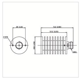
RF Solution offer a wide selection of Coaxial Fixed Termination (Dummy Load) for global customers. CT-30W-RA3857-NK-18G is a Coaxial Fixed Termination (Dummy Load) in Frequency Range of DC~18.0 GHz. It is made of high quality materials under a high standard, the Connector Type of this product is N-F (K), VSWR Max is 1.30 and Impedance is 50  $\Omega$ . The component has a good working performance and stability, it is ideal for handling a Power of 30 W.
