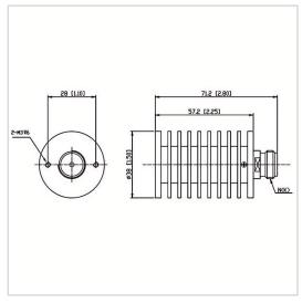
RF Solution offer a wide selection of Coaxial Fixed Termination (Dummy Load) for global customers. CT-30W-RA3857-NK-12.4G is a Coaxial Fixed Termination (Dummy Load) in Frequency Range of DC~12.4 GHz. It is made of high quality materials under a high standard, the Connector Type of this product is N-F (K), VSWR Max is 1.30 and Impedance is 50  $\Omega$ . The component has a good working performance and stability, it is ideal for handling a Power of 30 W.
