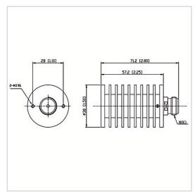
RF Solution offer a wide selection of Coaxial Fixed Termination (Dummy Load) for global customers. CT-30W-RA3857-NK-10G is Coaxial Fixed Termination (Dummy Load) in Frequency Range of DC~10.0 GHz. It is made of high quality materials under a high standard, the Connector Type of this product is N-F (K), VSWR Max is 1.30 and Impedance is 50  $\Omega$ . The component has a good working performance and stability, it is ideal for handling a Power of 30 W.
