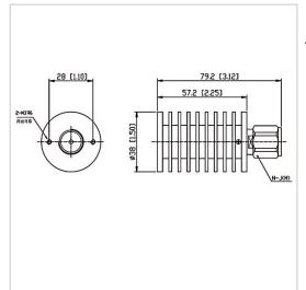
RF Solution offer a wide selection of Coaxial Fixed Termination (Dummy Load) for global customers. CT-30W-RA3857-NJ-8G is a Coaxial Fixed Termination (Dummy Load) in Frequency Range of DC~8.0 GHz. It is made of high quality materials under a high standard, the Connector Type of this product is N-M (J), VSWR Max is 1.30 and Impedance is 50  $\Omega$ . The component has a good working performance and stability, it is ideal for handling a Power of 30 W.
