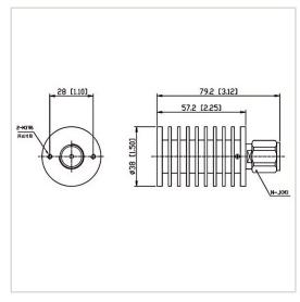
RF Solution offer a wide selection of Coaxial Fixed Termination (Dummy Load) for global customers. CT-30W-RA3857-NJ-6G is a Coaxial Fixed Termination (Dummy Load) in Frequency Range of DC $\sim$ 6.0 GHz. It is made of high quality materials under a high standard, the Connector Type of this product is N-M (J), VSWR Max is 1.25 and Impedance is 50  $\Omega$ . The component has a good working performance and stability, it is ideal for handling a Power of 30 W.
