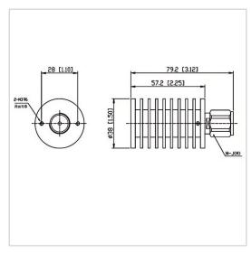
RF Solution offer a wide selection of Coaxial Fixed Termination (Dummy Load) for global customers. CT-30W-RA3857-NJ-4G is a Coaxial Fixed Termination (Dummy Load) in Frequency Range of DC $\sim$ 4.0 GHz. It is made of high quality materials under a high standard, the Connector Type of this product is N-M (J), VSWR Max is 1.20 and Impedance is 50  $\Omega$ . The component has a good working performance and stability, it is ideal for handling a Power of 30 W.
