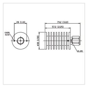
RF Solution offer a wide selection of Coaxial Fixed Termination (Dummy Load) for global customers. CT-30W-RA3857-NJ-3G is a Coaxial Fixed Termination (Dummy Load) in Frequency Range of DC~3.0 GHz. It is made of high quality materials under a high standard, the Connector Type of this product is N-M (J), VSWR Max is 1.20 and Impedance is 50  $\Omega$ . The component has a good working performance and stability, it is ideal for handling a Power of 30 W.
