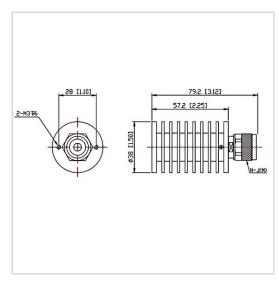
RF Solution offer a wide selection of Coaxial Fixed Termination (Dummy Load) for global customers. CT-30W-RA3857-NJ-10G is a Coaxial Fixed Termination (Dummy Load) in Frequency Range of DC~10.0 GHz. It is made of high quality materials under a high standard, the Connector Type of this product is N-M (J), VSWR Max is 1.30 and Impedance is 50  $\Omega$ . The component has a good working performance and stability, it is ideal for handling a Power of 30 W.
