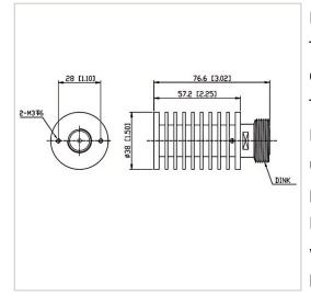
RF Solution offer a wide selection of Coaxial Fixed Termination (Dummy Load) for global customers. CT-30W-RA3857-DINK-6G is a Coaxial Fixed Termination (Dummy Load) in Frequency Range of DC~6.0 GHz. It is made of high quality materials under a high standard, the Connector Type of this product is DIN-F (K), VSWR Max is 1.25 and Impedance is 50  $\Omega$ . The component has a good working performance and stability, it is ideal for handling a Power of 30 W.
