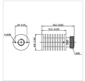
RF Solution offer a wide selection of Coaxial Fixed Termination (Dummy Load) for global customers. CT-30W-RA3857-DINK-3G is a Coaxial Fixed Termination (Dummy Load) in Frequency Range of DC~3.0 GHz. It is made of high quality materials under a high standard, the Connector Type of this product is DIN-F (K), VSWR Max is 1.20 and Impedance is 50  $\Omega$ . The component has a good working performance and stability, it is ideal for handling a Power of 30 W.
