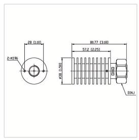
RF Solution offer a wide selection of Coaxial Fixed Termination (Dummy Load) for global customers. CT-30W-RA3857-DINJ-6G is a Coaxial Fixed Termination (Dummy Load) in Frequency Range of DC~6.0 GHz. It is made of high quality materials under a high standard, the Connector Type of this product is DIN-M (J), VSWR Max is 1.30 and Impedance is 50  $\Omega$ . The component has a good working performance and stability, it is ideal for handling a Power of 30 W.
