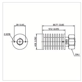
RF Solution offer a wide selection of Coaxial Fixed Termination (Dummy Load) for global customers. CT-30W-RA3857-DINJ-4G is a Coaxial Fixed Termination (Dummy Load) in Frequency Range of DC~4.0 GHz. It is made of high quality materials under a high standard, the Connector Type of this product is DIN-M (J), VSWR Max is 1.25 and Impedance is 50  $\Omega$ . The component has a good working performance and stability, it is ideal for handling a Power of 30 W.
