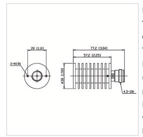
RF Solution offer a wide selection of Coaxial Fixed Termination (Dummy Load) for global customers. CT-30W-RA3857-4310K-6G is a Coaxial Fixed Termination (Dummy Load) in Frequency Range of DC~6.0 GHz. It is made of high quality materials under a high standard, the Connector Type of this product is 4.3-10-F (K), VSWR Max is 1.30 and Impedance is 50  $\Omega$ . The component has a good working performance and stability, it is ideal for handling a Power of 30 W.
