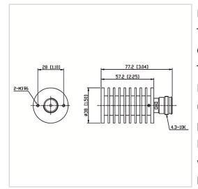
RF Solution offer a wide selection of Coaxial Fixed Termination (Dummy Load) for global customers. CT-30W-RA3857-4310K-4G is a Coaxial Fixed Termination (Dummy Load) in Frequency Range of DC~4.0 GHz. It is made of high quality materials under a high standard, the Connector Type of this product is 4.3-10-F (K), VSWR Max is 1.25 and Impedance is 50  $\Omega$ . The component has a good working performance and stability, it is ideal for handling a Power of 30 W.
