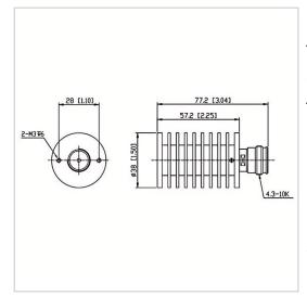
RF Solution offer a wide selection of Coaxial Fixed Termination (Dummy Load) for global customers. CT-30W-RA3857-4310K-3G is a Coaxial Fixed Termination (Dummy Load) in Frequency Range of DC~3.0 GHz. It is made of high quality materials under a high standard, the Connector Type of this product is 4.3-10-F (K), VSWR Max is 1.20 and Impedance is 50  $\Omega$ . The component has a good working performance and stability, it is ideal for handling a Power of 30 W.
