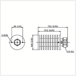
RF Solution offer a wide selection of Coaxial Fixed Termination (Dummy Load) for global customers. CT-30W-RA3857-4310J-6G is а Coaxial Termination (Dummy Load) in Frequency Range of DC~4.0 GHz. It is made of high quality materials under a high standard, the Connector Type of this product is 4.3-10-M (J), VSWR Max is 1.25 and Impedance is 50  $\Omega$ . The component has a good working performance and stability, it is ideal for handling a Power of 30 W.
