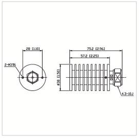
RF Solution offer a wide selection of Coaxial Fixed Termination (Dummy Load) for global customers. CT-30W-RA3857-4310J-3G is a Coaxial Fixed Termination (Dummy Load) in Frequency Range of DC~3.0 GHz. It is made of high quality materials under a high standard, the Connector Type of this product is 4.3-10-M (J), VSWR Max is 1.20 and Impedance is 50  $\Omega$ . The component has a good working performance and stability, it is ideal for handling a Power of 30 W.
