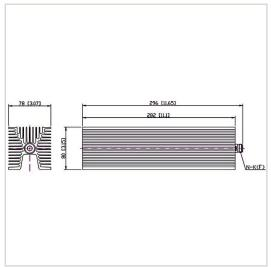
RF Solution offer a wide selection of Coaxial Fixed Termination (Dummy Load) for global customers. CT-300W-FA8028-NK-6G is a Coaxial Fixed Termination (Dummy Load) in Frequency Range of DC $\sim$ 6.0 GHz. It is made of high quality materials under a high standard, the Connector Type of this product is N-F (K), VSWR Max is 1.30 and Impedance is 50  $\Omega$ . The component has a good working performance and stability, it is ideal for handling a Power of 300 W.
