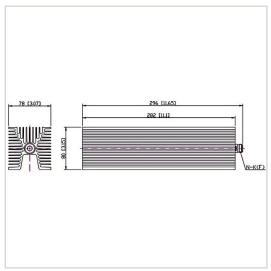
RF Solution offer a wide selection of Coaxial Fixed Termination (Dummy Load) for global customers. CT-300W-FA8028-NK-4G is a Coaxial Fixed Termination (Dummy Load) in Frequency Range of DC~4.0 GHz. It is made of high quality materials under a high standard, the Connector Type of this product is N-F (K), VSWR Max is 1.25 and Impedance is 50  $\Omega$ . The component has a good working performance and stability, it is ideal for handling a Power of 300 W.
