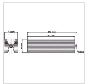
RF Solution offer a wide selection of Coaxial Fixed Termination (Dummy Load) for global customers. CT-300W-FA8028-NK-3G is a Coaxial Fixed Termination (Dummy Load) in Frequency Range of DC~3.0 GHz. It is made of high quality materials under a high standard, the Connector Type of this product is N-F (K), VSWR Max is 1.25 and Impedance is 50  $\Omega$ . The component has a good working performance and stability, it is ideal for handling a Power of 300 W.
