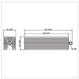
RF Solution offer a wide selection of Coaxial Fixed Termination (Dummy Load) for global customers. CT-300W-FA8028-NJ-6G is a Coaxial Fixed Termination (Dummy Load) in Frequency Range of DC $\sim$ 6.0 GHz. It is made of high quality materials under a high standard, the Connector Type of this product is N-M (J), VSWR Max is 1.30 and Impedance is 50  $\Omega$ . The component has a good working performance and stability, it is ideal for handling a Power of 300 W.
