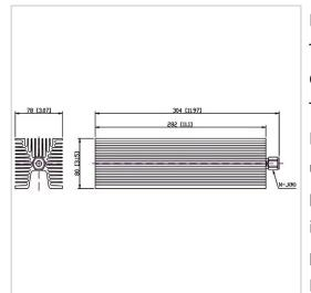
RF Solution offer a wide selection of Coaxial Fixed Termination (Dummy Load) for global customers. CT-300W-FA8028-NJ-4G is a Coaxial Fixed Termination (Dummy Load) in Frequency Range of DC~4.0 GHz. It is made of high quality materials under a high standard, the Connector Type of this product is N-M (J), VSWR Max is 1.25 and Impedance is 50  $\Omega$ . The component has a good working performance and stability, it is ideal for handling a Power of 300 W.
