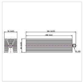
RF Solution offer a wide selection of Coaxial Fixed Termination (Dummy Load) for global customers. CT-300W-FA8028-NJ-3G is a Coaxial Fixed Termination (Dummy Load) in Frequency Range of DC $\sim$ 3.0 GHz. It is made of high quality materials under a high standard, the Connector Type of this product is N-M (J), VSWR Max is 1.25 and Impedance is 50  $\Omega$ . The component has a good working performance and stability, it is ideal for handling a Power of 300 W.
