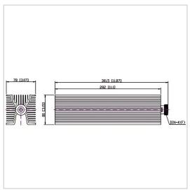
RF Solution offer a wide selection of Coaxial Fixed Termination (Dummy Load) for global customers. CT-300W-FA8028-DINK-6G is a Coaxial Fixed Termination (Dummy Load) in Frequency Range of DC~6.0 GHz. It is made of high quality materials under a high standard, the Connector Type of this product is DIN-F (K), VSWR Max is 1.30 and Impedance is 50  $\Omega$ . The component has a good working performance and stability, it is ideal for handling a Power of 300 W.
