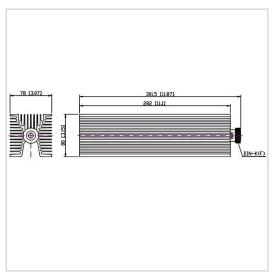
RF Solution offer a wide selection of Coaxial Fixed Termination (Dummy Load) for global customers. CT-300W-FA8028-DINK-3G is a Coaxial Fixed Termination (Dummy Load) in Frequency Range of DC $\sim$ 3.0 GHz. It is made of high quality materials under a high standard, the Connector Type of this product is DIN-F (K), VSWR Max is 1.25 and Impedance is 50  $\Omega$ . The component has a good working performance and stability, it is ideal for handling a Power of 300 W.
