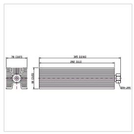
RF Solution offer a wide selection of Coaxial Fixed Termination (Dummy Load) for global customers. CT-300W-FA8028-DINJ-6G is a Coaxial Fixed Termination (Dummy Load) in Frequency Range of DC~6.0 GHz. It is made of high quality materials under a high standard, the Connector Type of this product is DIN-M (J), VSWR Max is 1.30 and Impedance is 50  $\Omega$ . The component has a good working performance and stability, it is ideal for handling a Power of 300 W.
