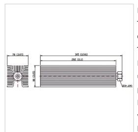
RF Solution offer a wide selection of Coaxial Fixed Termination (Dummy Load) for global customers. CT-300W-FA8028-DINJ-3G is a Coaxial Fixed Termination (Dummy Load) in Frequency Range of DC~3.0 GHz. It is made of high quality materials under a high standard, the Connector Type of this product is DIN-M (J), VSWR Max is 1.25 and Impedance is 50  $\Omega$ . The component has a good working performance and stability, it is ideal for handling a Power of 300 W.
