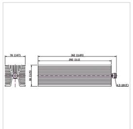
RF Solution offer a wide selection of Coaxial Fixed Termination (Dummy Load) for global customers. CT-300W-FA8028-4310K-6G is a Coaxial Fixed Termination (Dummy Load) in Frequency Range of DC~6.0 GHz. It is made of high quality materials under a high standard, the Connector Type of this product is 4.3-10-F (K), VSWR Max is 1.30 and Impedance is 50  $\Omega$ . The component has a good working performance and stability, it is ideal for handling a Power of 300 W.
