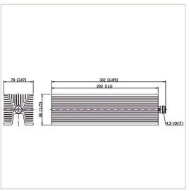
RF Solution offer a wide selection of Coaxial Fixed Termination (Dummy Load) for global customers. CT-300W-FA8028-4310K-3G is a Coaxial Fixed Termination (Dummy Load) in Frequency Range of DC~3.0 GHz. It is made of high quality materials under a high standard, the Connector Type of this product is 4.3-10-F (K), VSWR Max is 1.25 and Impedance is 50  $\Omega$ . The component has a good working performance and stability, it is ideal for handling a Power of 300 W.
