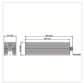
RF Solution offer a wide selection of Coaxial Fixed Termination (Dummy Load) for global customers. CT-300W-FA8028-4310J-6G is a Coaxial Fixed Termination (Dummy Load) in Frequency Range of DC~6.0 GHz. It is made of high quality materials under a high standard, the Connector Type of this product is 4.3-10-M (J), VSWR Max is 1.30 and Impedance is 50  $\Omega$ . The component has a good working performance and stability, it is ideal for handling a Power of 300 W.
