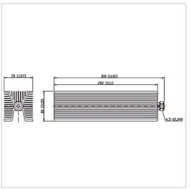
RF Solution offer a wide selection of Coaxial Fixed Termination (Dummy Load) for global customers. CT-300W-FA8028-4310J-4G is a Coaxial Fixed Termination (Dummy Load) in Frequency Range of DC~4.0 GHz. It is made of high quality materials under a high standard, the Connector Type of this product is 4.3-10-M (J), VSWR Max is 1.30 and Impedance is 50  $\Omega$ . The component has a good working performance and stability, it is ideal for handling a Power of 300 W.
