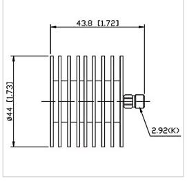
RF Solution offer a wide selection of Coaxial Fixed Termination (Dummy Load) for global customers. CT-20W-RA4434-2.92K-40G is a Coaxial Termination (Dummy Load) in Frequency Range of DC~40.0 GHz. It is made of high quality materials under a high standard, the Connector Type of this product is 2.92-F (K), VSWR Max is 1.30 and Impedance is 50  $\Omega$ . The component has a good working performance and stability, it is ideal for handling a Power of 20 W.
