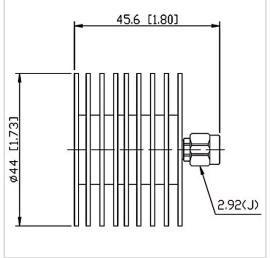
RF Solution offer a wide selection of Coaxial Fixed Termination (Dummy Load) for global customers. CT-20W-RA4434-2.92J-40G is a Coaxial Fixed Termination (Dummy Load) in Frequency Range of DC~40.0 GHz. It is made of high quality materials under a high standard, the Connector Type of this product is 2.92-M (J), VSWR Max is 1.30 and Impedance is 50  $\Omega$ . The component has a good working performance and stability, it is ideal for handling a Power of 20 W.
