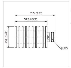
RF Solution offer a wide selection of Coaxial Fixed Termination (Dummy Load) for global customers. CT-20W-RA3657-NK-6G is a Coaxial Fixed Termination (Dummy Load) in Frequency Range of DC~6.0 GHz. It is made of high quality materials under a high standard, the Connector Type of this product is N-F (K), VSWR Max is 1.20 and Impedance is 50  $\Omega$ . The component has a good working performance and stability, it is ideal for handling a Power of 20 W.
