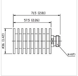
RF Solution offer a wide selection of Coaxial Fixed Termination (Dummy Load) for global customers. CT-20W-RA3657-NK-4G is Coaxial Fixed а Termination (Dummy Load) in Frequency Range of DC~4.0 GHz. It is made of high quality materials under a high standard, the Connector Type of this product is N-F (K), VSWR Max is 1.20 and Impedance is 50  $\Omega$ . The component has a good working performance and stability, it is ideal for handling a Power of 20 W.
