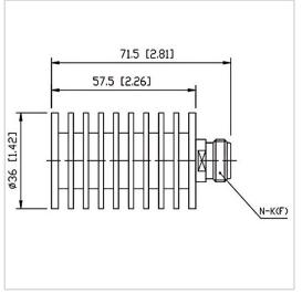
RF Solution offer a wide selection of Coaxial Fixed Termination (Dummy Load) for global customers. CT-20W-RA3657-NK-3G is Coaxial Fixed а Termination (Dummy Load) in Frequency Range of DC~3.0 GHz. It is made of high quality materials under a high standard, the Connector Type of this product is N-F (K), VSWR Max is 1.20 and Impedance is 50  $\Omega$ . The component has a good working performance and stability, it is ideal for handling a Power of 20 W.
