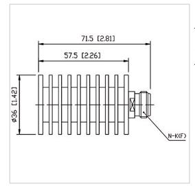
RF Solution offer a wide selection of Coaxial Fixed Termination (Dummy Load) for global customers. CT-20W-RA3657-NK-10G is a Coaxial Fixed Termination (Dummy Load) in Frequency Range of DC~10.0 GHz. It is made of high quality materials under a high standard, the Connector Type of this product is N-F (K), VSWR Max is 1.25 and Impedance is 50  $\Omega$ . The component has a good working performance and stability, it is ideal for handling a Power of 20 W.
