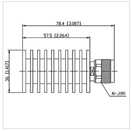
RF Solution offer a wide selection of Coaxial Fixed Termination (Dummy Load) for global customers. CT-20W-RA3657-NJ-8G is a Coaxial Fixed Termination (Dummy Load) in Frequency Range of DC~8.0 GHz. It is made of high quality materials under a high standard, the Connector Type of this product is N-M (J), VSWR Max is 1.20 and Impedance is 50  $\Omega$ . The component has a good working performance and stability, it is ideal for handling a Power of 20 W.
