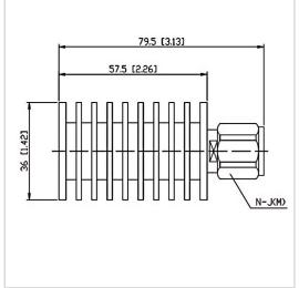
RF Solution offer a wide selection of Coaxial Fixed Termination (Dummy Load) for global customers. CT-20W-RA3657-NJ-6G is a Coaxial Fixed Termination (Dummy Load) in Frequency Range of DC~6.0 GHz. It is made of high quality materials under a high standard, the Connector Type of this product is N-M (J), VSWR Max is 1.25 and Impedance is 50  $\Omega$ . The component has a good working performance and stability, it is ideal for handling a Power of 20 W.
