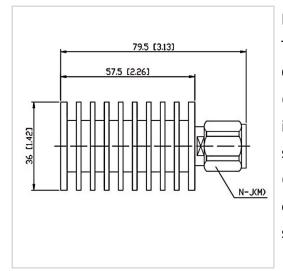
RF Solution offer a wide selection of Coaxial Fixed Termination (Dummy Load) for global customers. CT-20W-RA3657-NJ-3G is a Coaxial Fixed Termination (Dummy Load) in Frequency Range of DC $\sim$ 3.0 GHz. It is made of high quality materials under a high standard, the Connector Type of this product is N-M (J), VSWR Max is 1.20 and Impedance is 50  $\Omega$ . The component has a good working performance and stability, it is ideal for handling a Power of 20 W.
