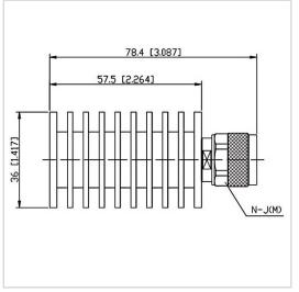
RF Solution offer a wide selection of Coaxial Fixed Termination (Dummy Load) for global customers. CT-20W-RA3657-NJ-18G is Coaxial Fixed а Termination (Dummy Load) in Frequency Range of DC~18.0 GHz. It is made of high quality materials under a high standard, the Connector Type of this product is N-M (J), VSWR Max is 1.30 and Impedance is 50  $\Omega$ . The component has a good working performance and stability, it is ideal for handling a Power of 20 W.
