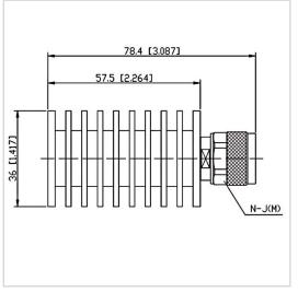
RF Solution offer a wide selection of Coaxial Fixed Termination (Dummy Load) for global customers. CT-20W-RA3657-NJ-12.4G is a Coaxial Fixed Termination (Dummy Load) in Frequency Range of DC~12.4 GHz. It is made of high quality materials under a high standard, the Connector Type of this product is N-M (J), VSWR Max is 1.25 and Impedance is 50  $\Omega$ . The component has a good working performance and stability, it is ideal for handling a Power of 20 W.
