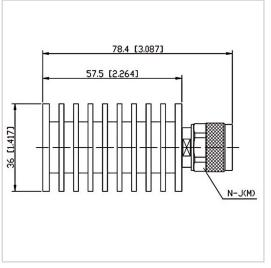
RF Solution offer a wide selection of Coaxial Fixed Termination (Dummy Load) for global customers. CT-20W-RA3657-NJ-10G is Coaxial Fixed а Termination (Dummy Load) in Frequency Range of DC~10.0 GHz. It is made of high quality materials under a high standard, the Connector Type of this product is N-M (J), VSWR Max is 1.25 and Impedance is 50  $\Omega$ . The component has a good working performance and stability, it is ideal for handling a Power of 20 W.
