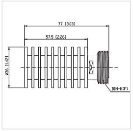
RF Solution offer a wide selection of Coaxial Fixed Termination (Dummy Load) for global customers. CT-20W-RA3657-DINK-6G is a Coaxial Fixed Termination (Dummy Load) in Frequency Range of DC~6.0 GHz. It is made of high quality materials under a high standard, the Connector Type of this product is DIN-F (K), VSWR Max is 1.30 and Impedance is 50  $\Omega$ . The component has a good working performance and stability, it is ideal for handling a Power of 20 W.
